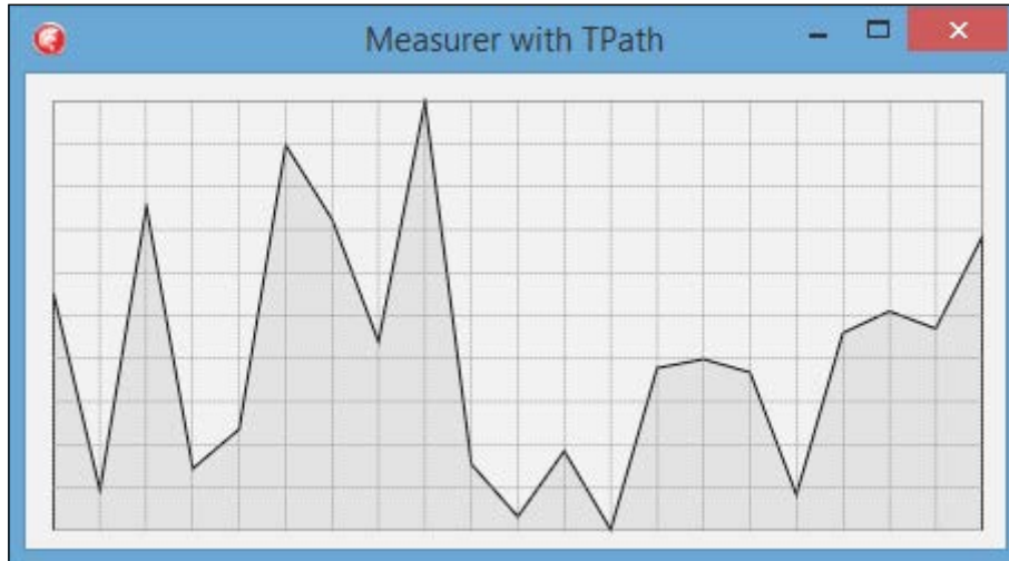
Scrolling data in a line graph; new data are pushed from the right-hand side and old data are removed from the left-hand side
